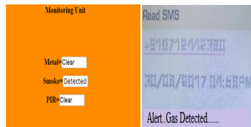
Figure 15 : Updates the webpage smoke sensor detected and GSM output
